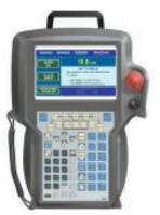
The WeldSaver graphical user Interface provides information on device status in real time, with clear visual indicators and descriptions. The interface can be accessed over a network using most JavaScript<sup>TML</sup> enabled web browsers by entering the working IP address of the device.
