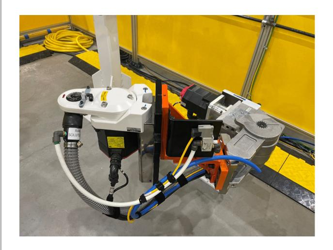
Fanuc Servo Motor with Brake option
