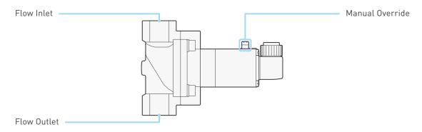
The solenoid valve controls the flow of water through the WeldSaver. When power is applied to the valve, it opens to allow water to pass through; when power is switched off, the valve automatically closes and thereby stops the flow of water.
