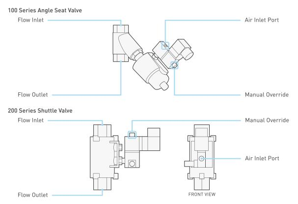
Both pneumatic valve assemblies are composed of small solenoid valve that controls the flow of compressed air to a larger pneumatic valve.
