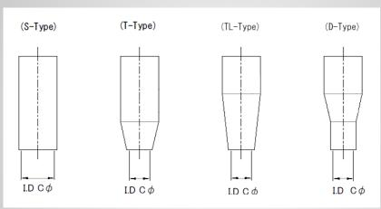
Please check the contact tip size and see if it will fit into reamer by checking "Reamer I.D"
