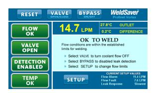
The WeldSaver graphical user interface provides information on device status in real time, with clear visual indicators and descriptions. The interface can be accessed over a network using most JavaScript™-enabled web browsers by entering the working IP address of the device.
