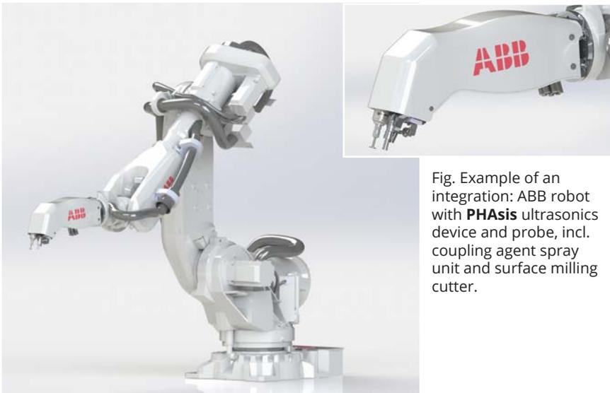
Fig. Example of an integration: ABB robot with **PHAsis** ultrasonics device and probe, incl. coupling agent spray unit and surface milling cutter.
